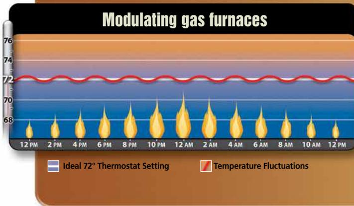
The Coleman® Echelon™ modulating gas furnace has been designed to maintain your ideal temperature by modulating heating level in .50 or .65% increments to match the degree of comfort you need precisely. Comfort is dramatically increased as the furnace adjusts its level of operation up or down to offset the rate at which heat leaves your home.
